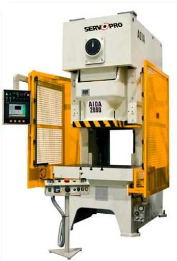
A single servo press can perform work that formerly required multiple machines, eliminating time-consuming pauses in the production cycle.
