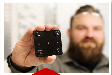
Jayson Marcott designed the tooling solution for this four-nut backing plate used on a refrigeration unit hinge.
